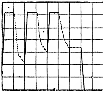
Fig. 37. Fatigue and reversal in the Ag' receiver. Thick lines represent the effect of radiation, and dotted lines the recovery. Observe in the first three records the incomplete recovery and increasing fatigue. In the fourth, there is produced a reversal (a diminution of resistance instead of the normal increase).
